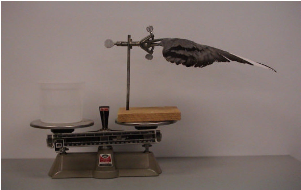
Figure 2. Mounted wing on balance with equal weight of water.
